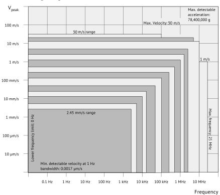
$<sup>^{*2}</sup>$  Velocity limited to 1 m/s at frequencies above 10 MHz.
